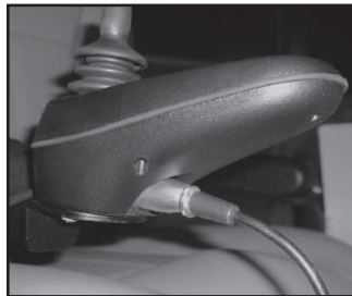
Off-board charger port (located under joystick)
